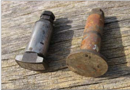
Curved shoe of "splasher" tappet versus round, flat shoe of StepDown tappet
